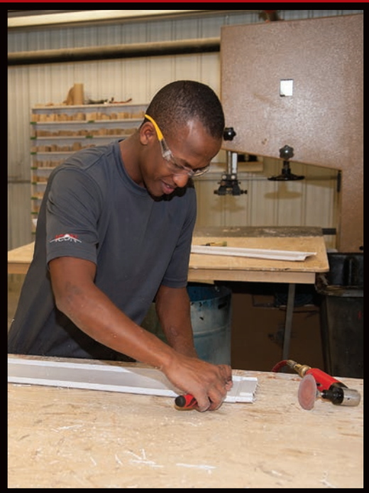
An ICON worker does trimming and detailing on a fender skirt, an initial step prior to the painting and packaging of the product. ICON has been particularly successful selling RV exterior replacement products no longer supported by RV manufacturers.
